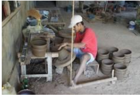
Figure 7. Oblique spinning technique
