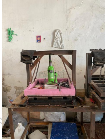
Gambar 52. Proses pressing cacahan plastik (Sumber: Khansa, 2024)
