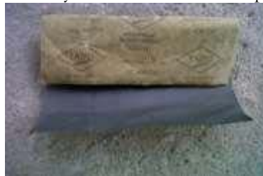
Picture. 6 The sandpaper used makes the dents
