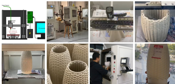
Figure 6. 3D printing experimental process.
