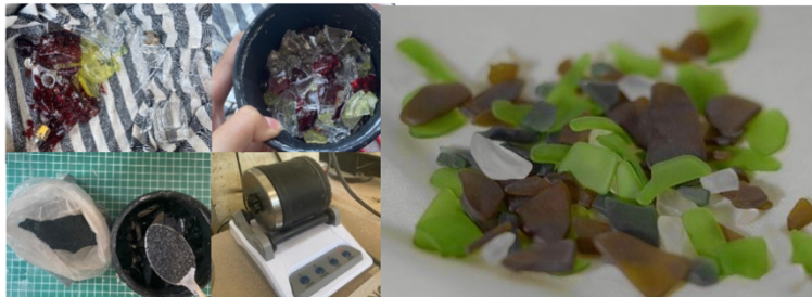
Figure 2. Processing Sea Glass with a tumbler rock glass Source: Author's Processing, 2024.
