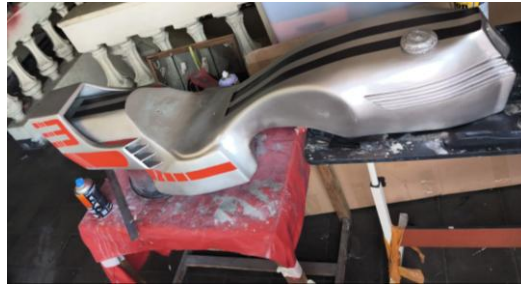
Gambar 4.53 Proses Decal Body
