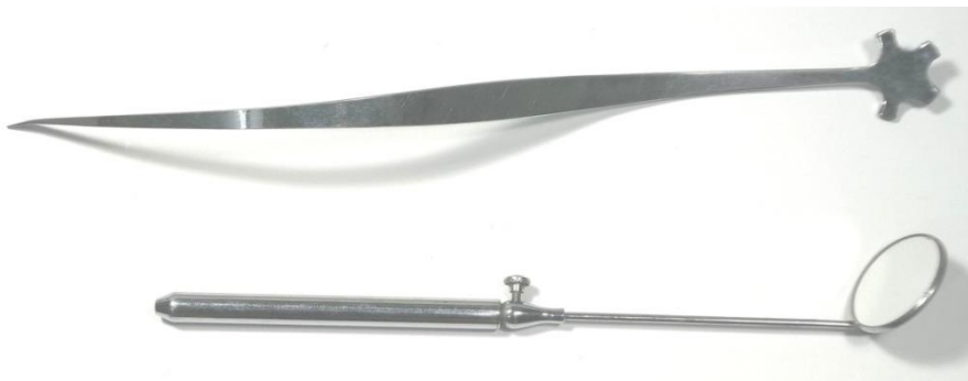
Gambar 4. Alat untuk memasang Sound-post ( Sound Post Setter dan Inspection mirror to control the soundpost setting ) (Foto: Kristiyanto, 2012)
